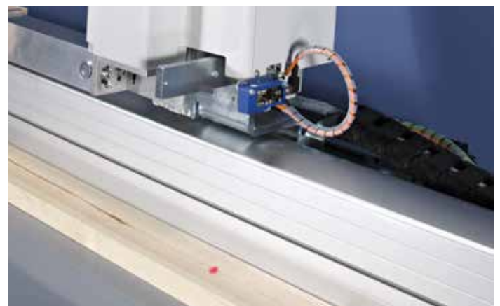
Close-up of pusher with workpiece measurement sensor
